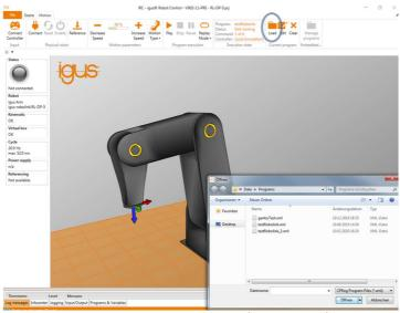
Figure 7.9 Loading a new program (marked in blue).
