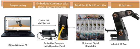
Figure 9.1: robolink DP with Embedded Computer as Robot Control
