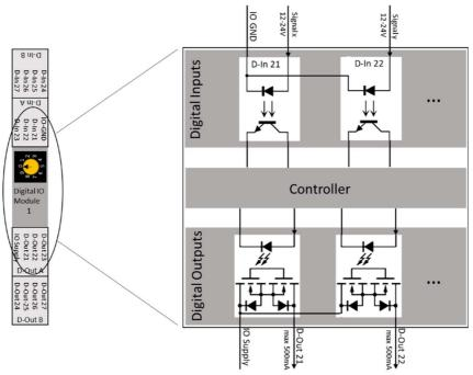
Figure 4.2: Internal set up of a DIO module
