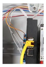
The 2 leaded ribbon cable of the Embedded Computer is the RS232 connection for the Operating Panel. One lead is marked black (lead 1).
