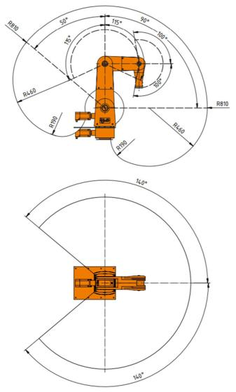
Figure 3.3 Schematic of operating range of igus® robolink® DP, 5-axis version.
