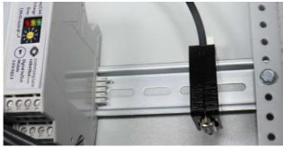
Figure 4.7: D-Sub connector to the Operating panel
