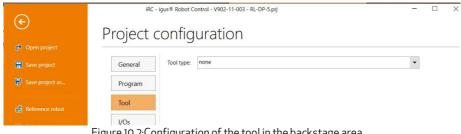
Figure 10.2: Configuration of the tool in the backstage area.
