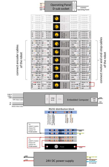
Figure 4.1 Overview of electrical connections.
