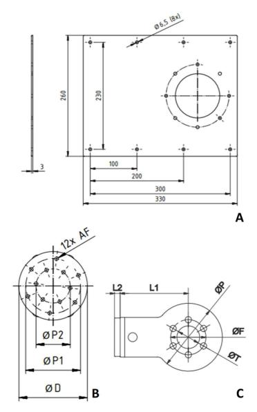
Figure 3.4 igus® robolink® DP of: A) Robot base; B), hole pattern flange of the 5<sup>th</sup> axis (five axes version); C) Gripper adapter (four axes version). Dimensions are depicted in mm.
