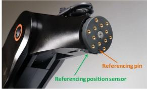
Figure 7.4 Referencing tools of Axis 5.
