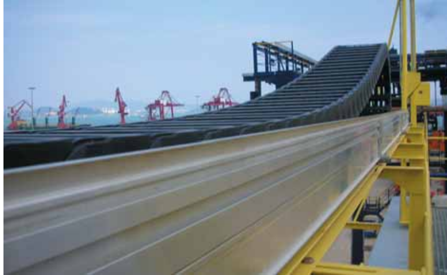
Super Alu Guide Trough – installed on a RTG-application
