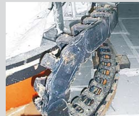
Sicherer Betrieb auch in schmutzigen Umgebungen Safe operation also in dirty environments - the robust link design allows safe work in a dirty environment
